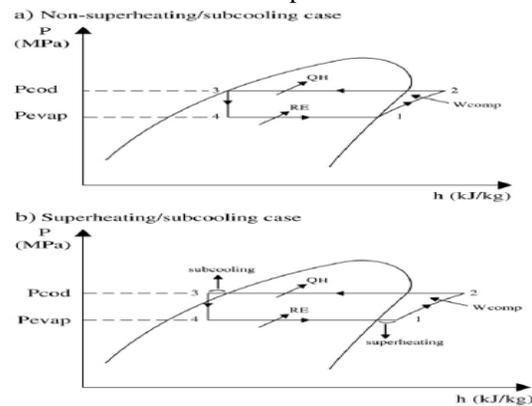
Fig.1 Tradition vapour-compression refrigeration cycle used in the analysis for the cases of (a) non-
