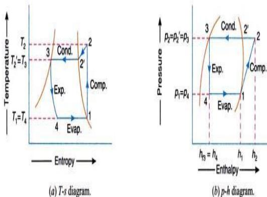
Fig: 3 T-S and P-H Diagram
