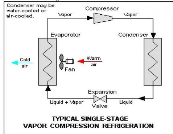
**Fig: 2 Block Diagram of Vapour Compression Refrigeration System**
