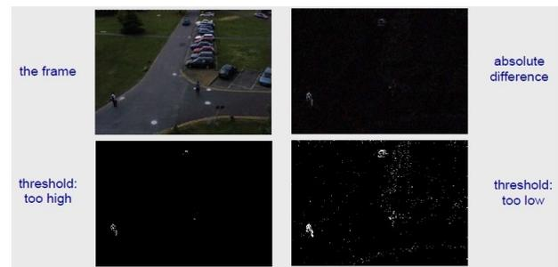
Frame difference results with Thresholds set at high and low.
