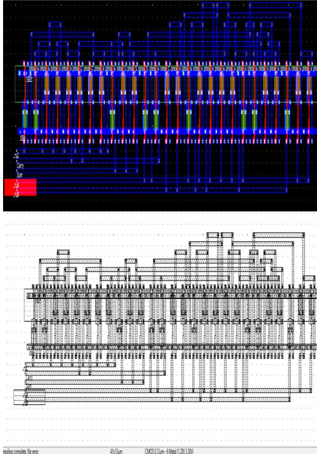
Figure 5 Layout of Proposed Full Adder Design in Micro-wind
