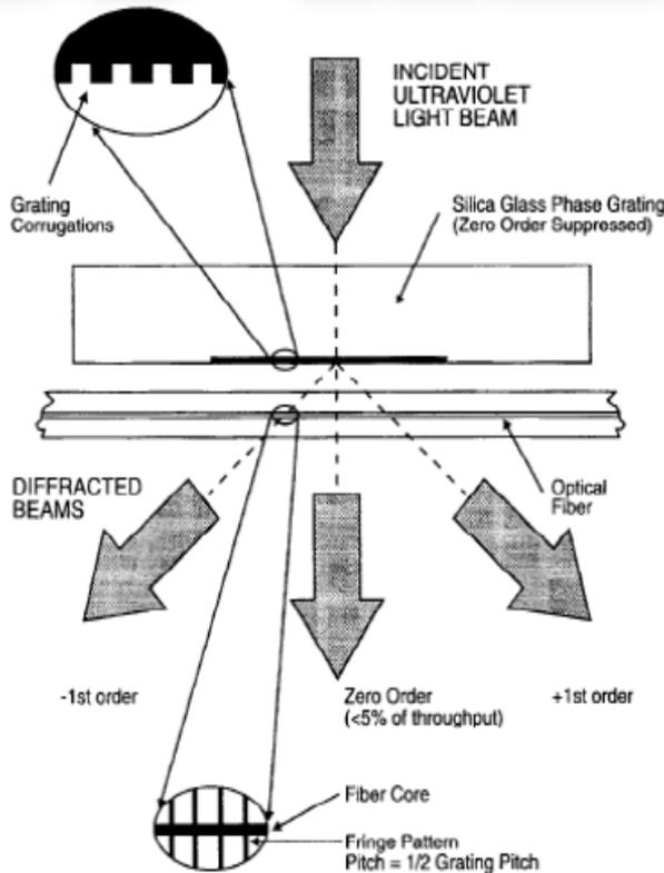
Figure 1: Bragg grating fabrication apparatus based on a zero-order nulled diffraction phase mask [1]
