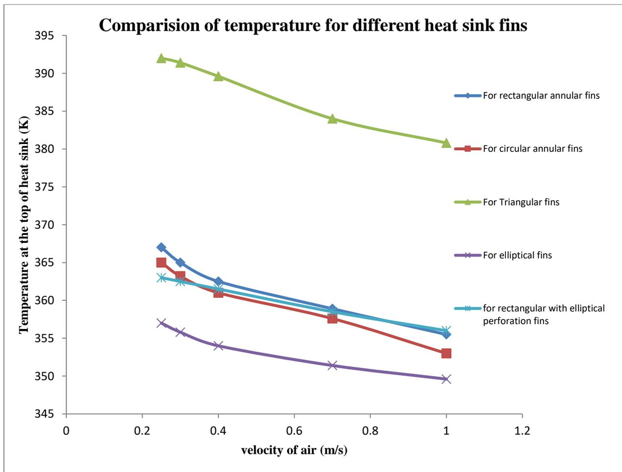
Figure 2: shows the comparison of temperature at the top of the heat sink using PLA as a working material for heat sink having different fins profile
