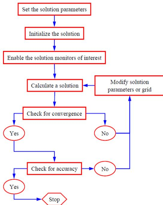
Figure 1: Flow chart for solution setup
