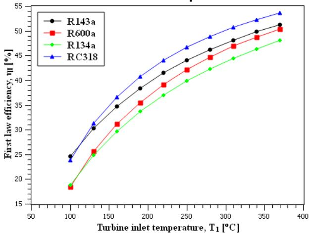
Figure 7: Variation Of First Law Efficiency Vs Turbine Inlet Temperature.
