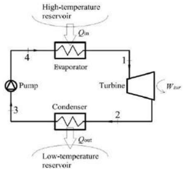
Figure 3: Schematic diagram of the organic Rankine cycle.
