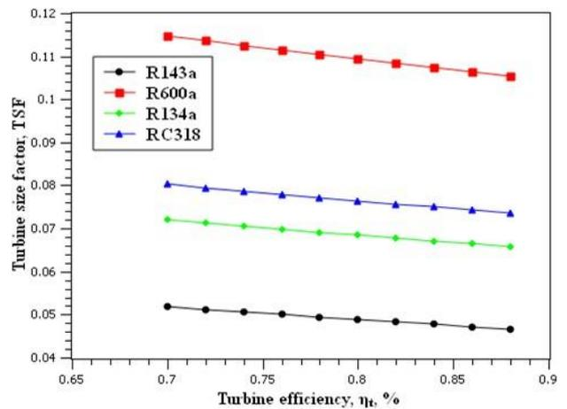
Figure 15: Variation of turbine size factor vs turbine efficiency.
